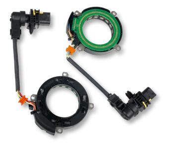
The Multi-Coil Resolver (MCR) is designed to determine synchronous electric motor rotor position by scanning magnetic fields. This MCR can withstand rotation speeds above 20,000 RPM and operates in a temperature range within -40°C up to +150°C. Depending on the various specifications, specific adaptations may increase these values.
