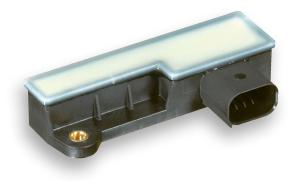
Industry Automotive Application Transmission, Brake, Clutch, Steering, Engine Functions Measuring travel or angle position Technology Active PLCD (moving magnet) Features • Measurement range 25-53mm • Highly insensitive to vibration • Temperature up to 150°C
