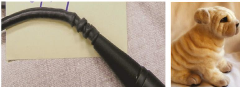
Fig.4. "Shar Pei" effect—stretching of cable jackets due to repeated manual cleaning
