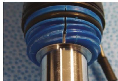
Fig.1. Mechanical stresses, like threaded mating components, can increase likelihood of cracking due to reprocessing.
