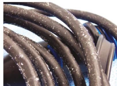
Fig.3. Blooming of Additives after repeated  $H_2O_2$  Sterilization.
