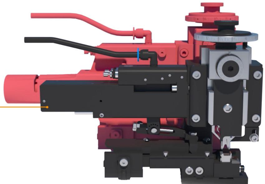
Smaller air feed design on the OCEAN 2.0 Applicator fits into more terminators
