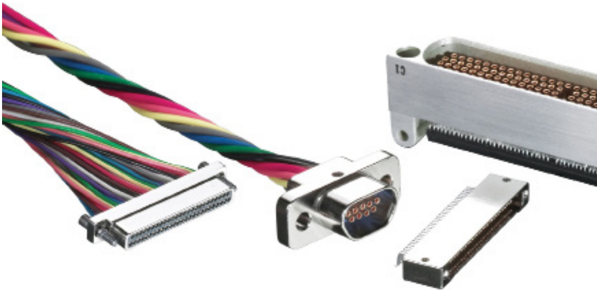
FIGURE 4. NANOMINIATURE CONNECTORS (LEFT AND LOWER RIGHT) OFFER EXTREME REDUCTIONS IN SIZE AND WEIGHT COMPARED TO MICROD CONNECTORS. (SOURCE: TE CONNECTIVITY)
