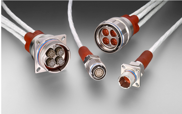
Figure 1: Example of 38999 Series III-style acme threaded connectors that support 10 Gb/s Ethernet and higher. (CeeLok FAS-X connectors provided by TE Connectivity.)
