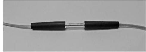
LightCrimp splices provide rugged, miniaturized form-factor that assures consistent crimp quality, dependability, and performance that rivals fusion splices. LightCrimp splices have been tested in accordance with IEC 61300 procedures, with an operating temperature range extending from -25° C to +70° C.
