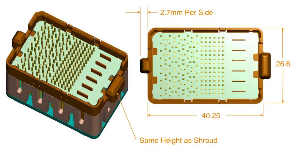
Guideposts allow up to approximately 2mm offset for blindmating
