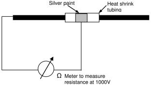
N.B. ensure inside of metal tube is clean and a good electrical contact is achieved.
