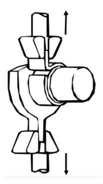
Figure 2. Part Specimen in Tensile Tester – (Rolling Drum Method Illustrated)
