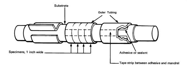
Figure 1. Peel Specimen Preparation
