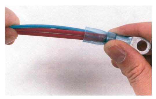
Equip the hot air gun with the reflector and then allow it to warm up until the operating temperature is reached (See paragraph 2)
