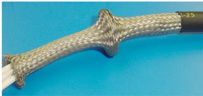
Figure 5. Bunching the Braided Shield
