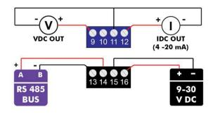
LVDT/LVRT Connection Diagram
