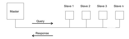
In the MODBUS protocol the master can address individual slaves, or, using a special "Broadcast" address, can initiate a broadcast message to all slaves. The Integra products do not support the broadcast address.
