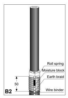
Bind and solder the earth braid to the metal tape shield (or attach the earth lead by any other equivalent method). Fill the earth braid with solder to form a 30 mm moisture block 20 mm from the oversheath end.
