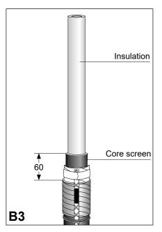
Thoroughly remove the core screen to within 60 mm of the oversheath cut. The surface of the insulation should be free from all traces of conductive material.
