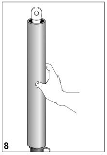
Preheat the cable lug slightly before placing the tubing over the core. The bottom end of the tubing should be level with the wire binder.
