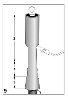
Shrink the tubing down starting at the screen cut **using a soft yellow flame**. Heat the area well but avoid scorching of surface. Continue shrinking towards the cable lug.
