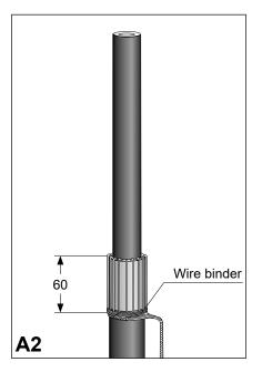
Bend the shielding wires back onto the oversheath. Avoid crossing the individual wires.
