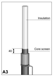
Thoroughly remove the core screen to within 40 mm of the oversheath cut. The surface of the insulation should be free from all traces of conductive material.
