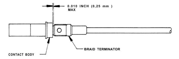
• The solder must have completely melted and flowed through the holes in the braid terminator body and into the braid strands underneath.
