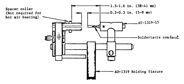
Figure 4: **Set-Up Dimension for AD-1319 Holding Fixture**
