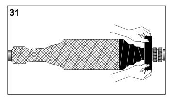
Remove the insulation on the earth leads for 120 mm. Spread the wires and position the wires onto the copper braids close to the oversheath cut. Fix the earth leads with a worm drive clamp on both sides.
