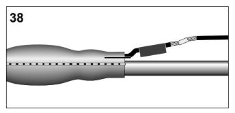
Position the insulating tubing centrally over the connector and shrink down starting in the center working towards the ends.
