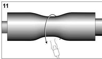
Smooth out the step at the tubing end with PVC tape.
