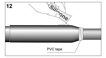
Push the main body on the tubing in a parking position. In doing so, twist the main body in order to spread the silicone grease evenly under the main body.
