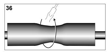
Place the wraparound centrally over the shrunk tubes. Close it at the metal channel.
