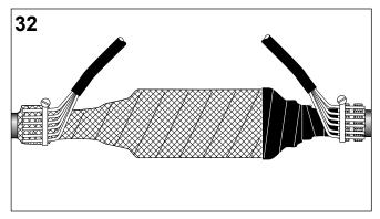
Fold the earth leads back over the worm drive clamp and apply a second worm drive clamp.
