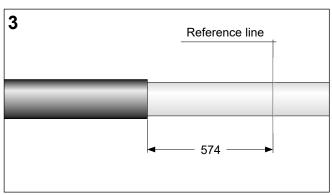
Remove the metal tape 100 mm from the oversheath cut.
