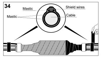
Slide one of the two sleeves centrally over the joint. Shrink the tubing down, starting in the center working towards the ends.
