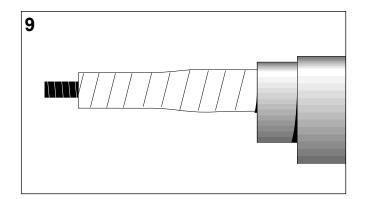
Slide the tube (short) onto the other cable as shown in the drawing.
