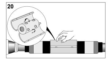
Apply conductive self-amalgamating tape onto the black part of the adapter and conductive cable screen on both ends, see drawing.
