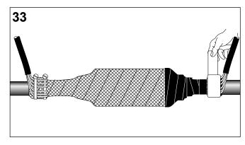
Slightly lift the shield wires.
