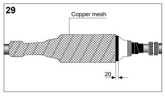
Apply non-conductive tape with at least 5 mm thickness onto the visible part of the adapter and main body as shown. Start 10 mm on the conductive part of the adapter and stop 20 mm on the semi-conductive part of the main body.
