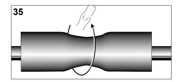
Slide the second sleeve centrally over the joint. Shrink the tubing down, starting in the center working towards the ends.
