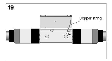
Install the Faraday cage (see detail) and make sure the step from the cable insulation to the Faraday cage does not exceed 2 mm.
