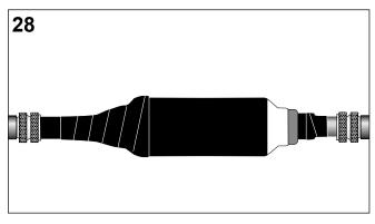
Wrap one layer of tinned copper mesh with a 50% overlap around the joint as shown. Start wrapping on the metal tape. Stop 20 mm before the semi-conductive area of main body ends.
