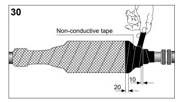
Smooth out the step between self-amalgamating tape and the sheath cut with black mastic tape.
