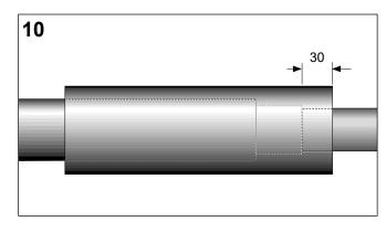
Start shrinking in the middle of the tubing and shrink it completely down.
