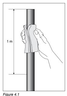
**4.1**. Clean and degrease the end of the oversheath for a length of 1 meter with solvent wipe.
