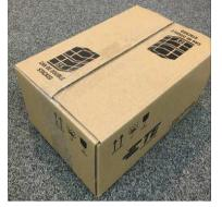
After Test: Carton dropping corner and edge were out of shape. Inner packaging was OK. Products were OK.
