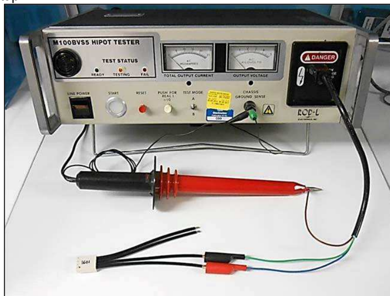
FIGURE 10 – DIELECTRIC BREAKDOWN TEST SETUP
