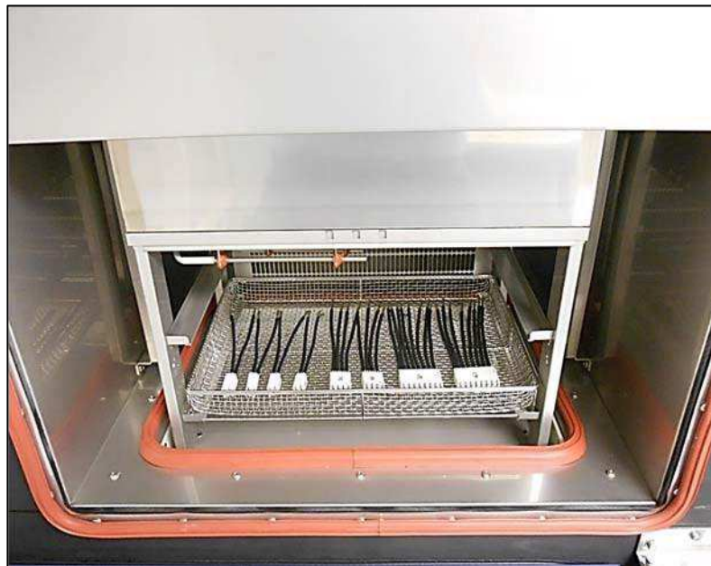
FIGURE 4 – THERMAL SHOCK TEST SETUP
