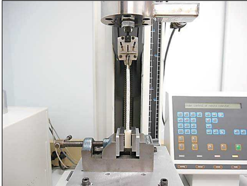
Figure 9 – Contact Retention Force Test Setup
