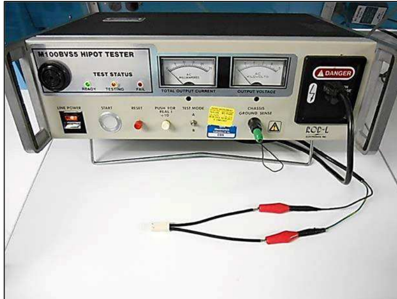
Figure 3 – DWV Test Setup
