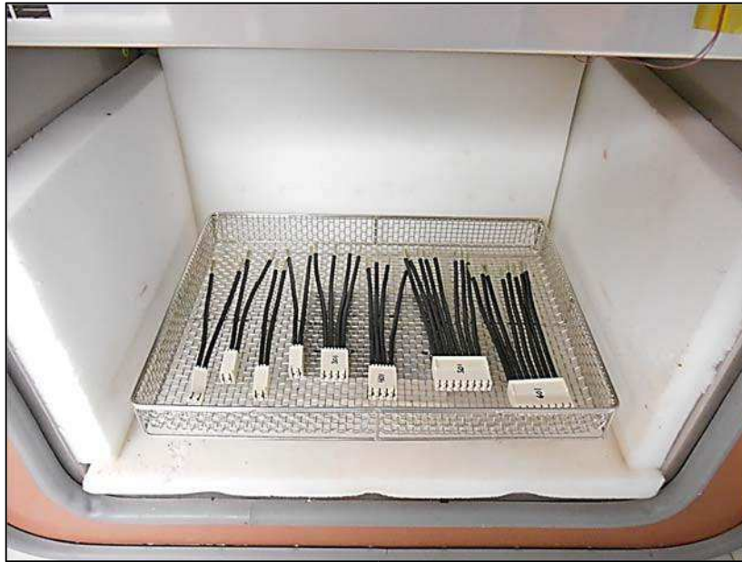
Figure 7 – Low Temperature Test Setup
