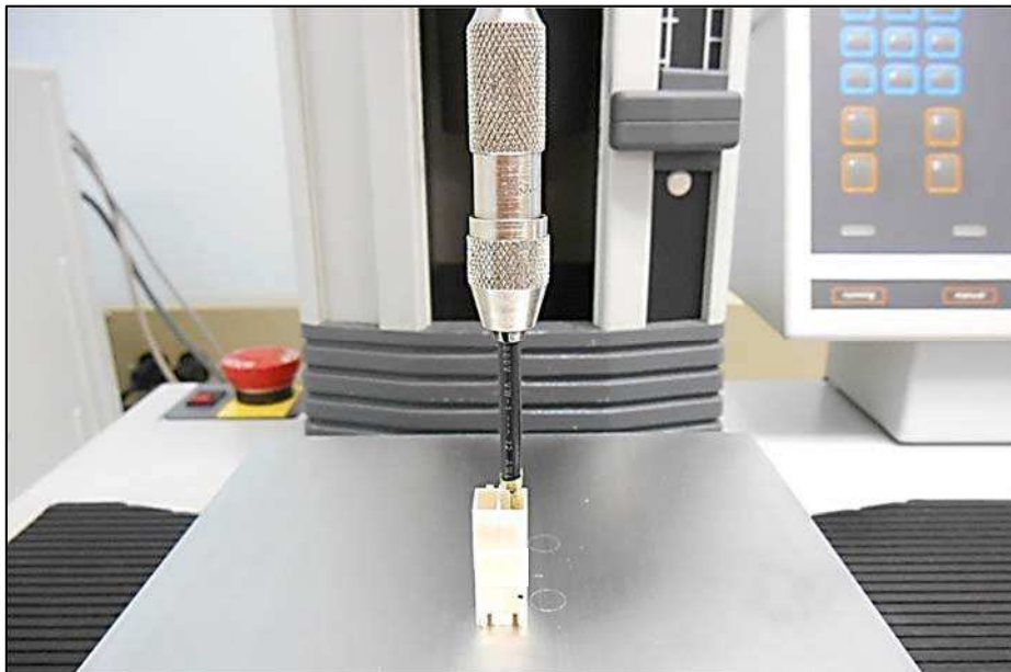
FIGURE 8 – CONTACT INSERTION FORCE TEST SETUP
