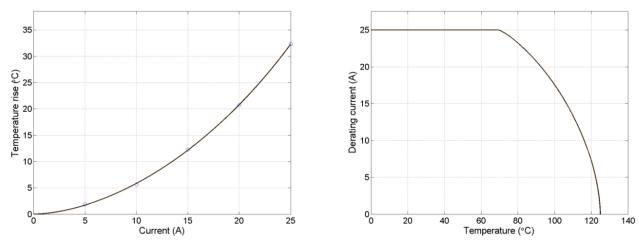
Fig 4: 2238196-3 AWG14# Derating Curve
