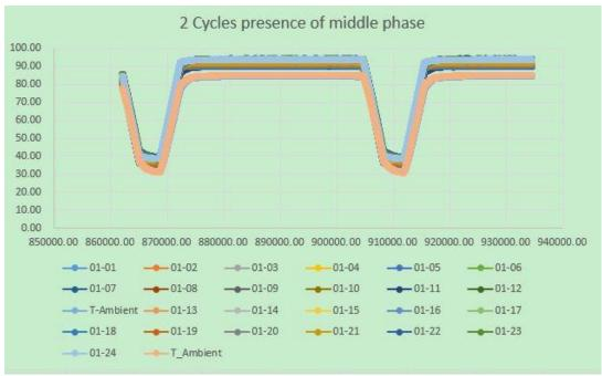
Fig.2: Temperature on specimens data example of 2 cycles when test run half
