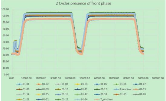
Fig.1: Temperature on specimens data example of 2 cycles when test start
