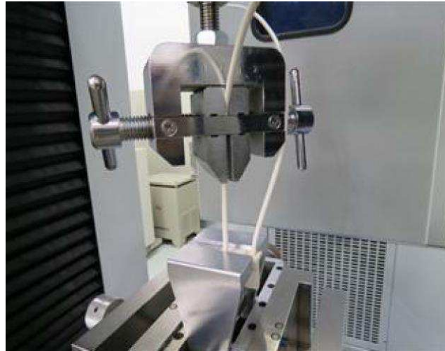
Figure – 6 typical retention force setups
