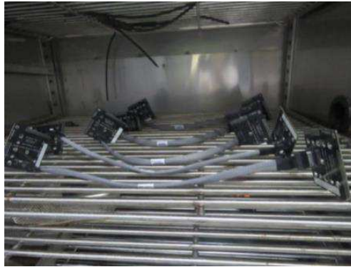
Figure 9 – Damp Heat Steady State Test Setup
