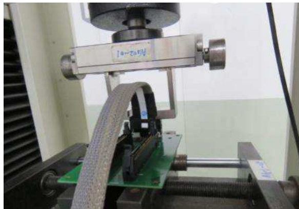
Figure 6 – Mating Force Test Setup
