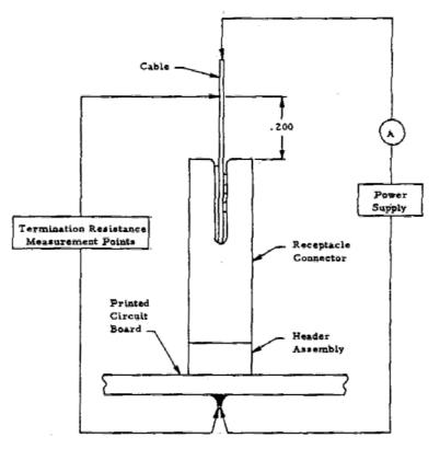
Figure 4 Typical Termination Resistance Measurement Points
