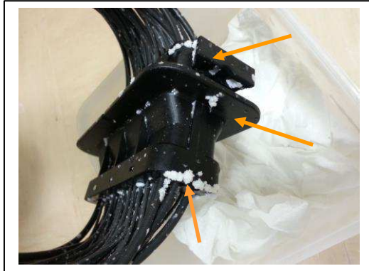
Figure 10: Fluid Resistance test: ADBLUE, formation of Urea crystals on part as water evaporates from ADBLUE solution during 24 Hour air dry cycles.
