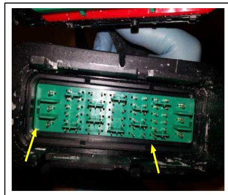
Figure 11: No Urea crystals on mating surface of part
