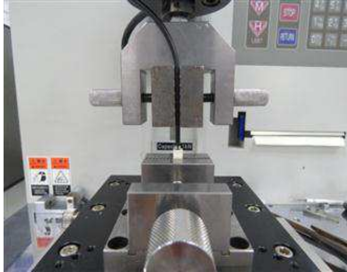
Figure 5 – typical contact insertion force setup
