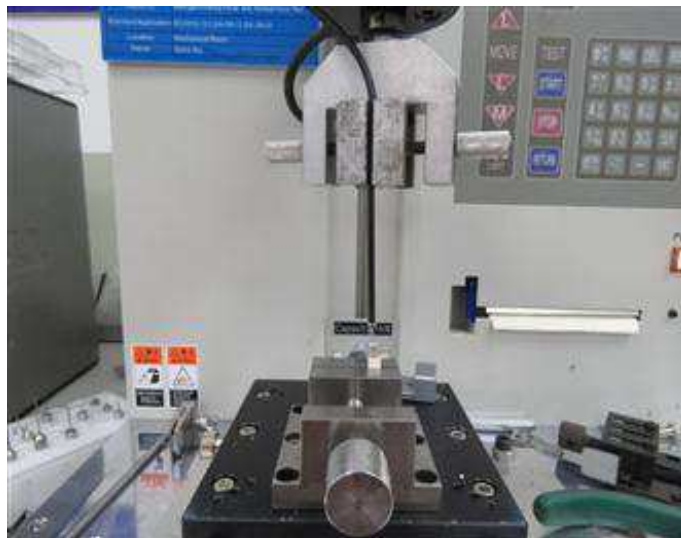
Figure – 6 typical retention force setups
