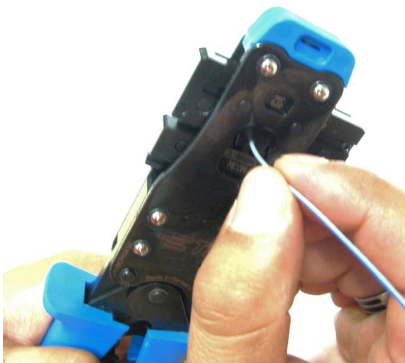
Figure 4: Crimp terminal (left), check the crimped terminal (right)
