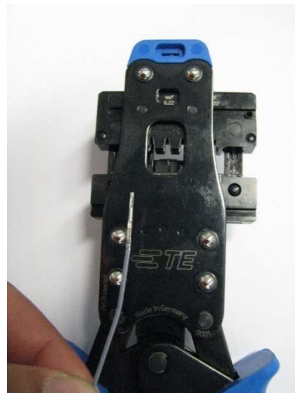
Figure 4: Crimp terminal (left), check the crimped terminal (right)
