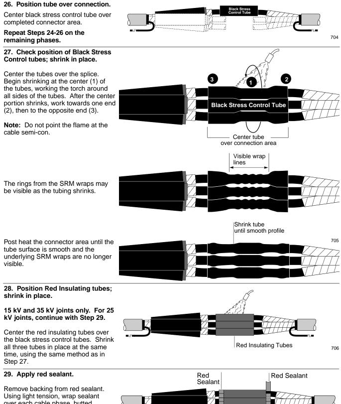
Using light tension, wrap sealant over each cable phase, butted against the tubes as shown. Build the sealant to the level of the previously installed tube.
