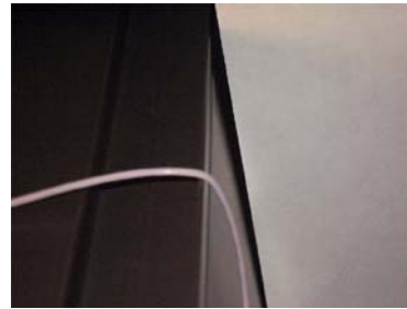
DO NOT Allow Twist in Fiber Optic Cable
