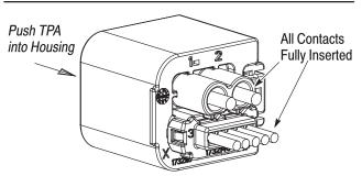
Note: Assembly –1 Shown Assembly –2 Only Accepts 4 Signal Contacts
