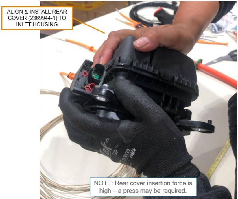
Figure 60: Rear cover installation
