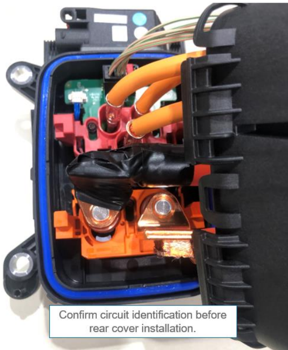
Figure 59: Proper circuit identification before rear cover installation
