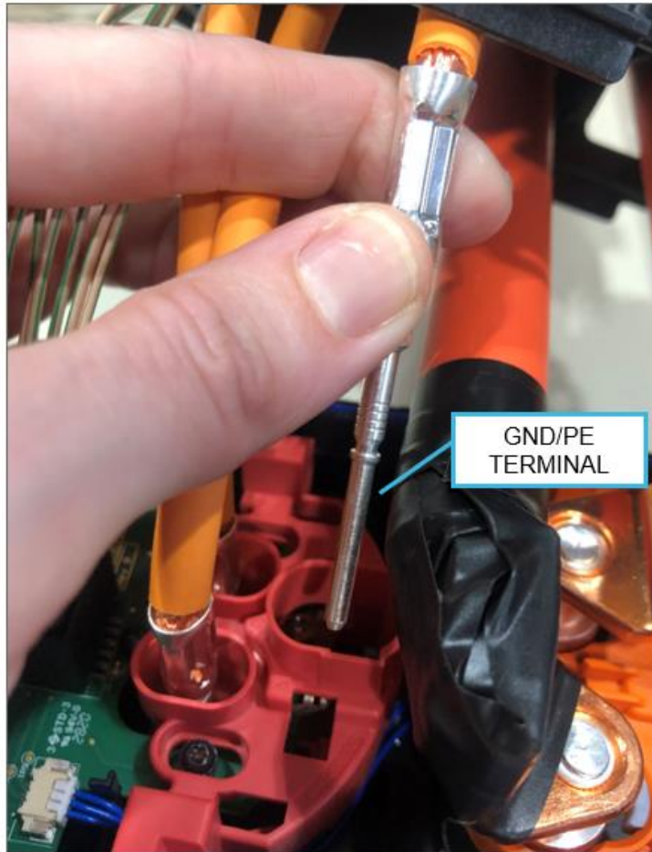
Figure 53: GND/PE Terminal installation into inlet assembly
