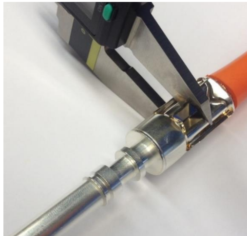
Figure 13: Digital caliper positioning on processed crimp (exemplary image)
