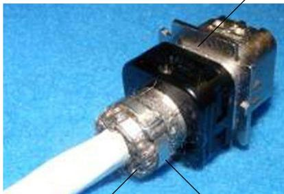
All Cable Shields Folded Over Cable Exit Halves
