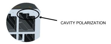
• INSERT THE TERMINAL UNTIL AN AUDIBLE "CLICK" IS HEARD OR THE LOCK IS FELT WHEN THE TERMINAL LANCE HAS ENGAGED INTO RELEVANT CARRIER HOUSING LOCKING HOLE.
