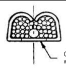
Cutoff tab centered with centerline of splice within 0.38 [.015] TIR.
