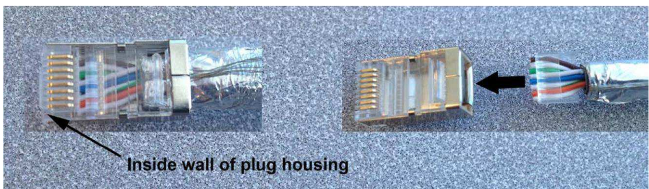
Figure 2-5: Insert the wired load bar into plug
