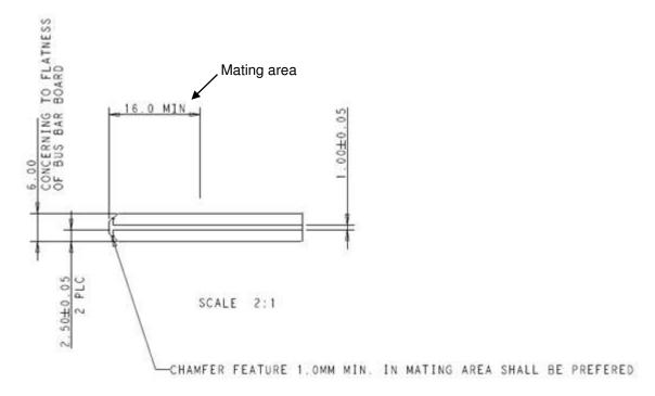
Figure 3. Laminated Mating Bus Bar Board View.
