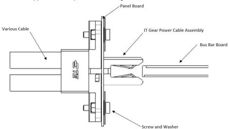
Figure 4. Visual Aid of TE Connectivity OCP IT Gear Power Cable Assembly
