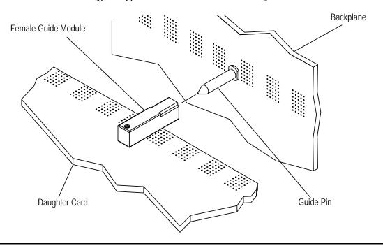
Typical Applied Guide Module and Pin Assembly
