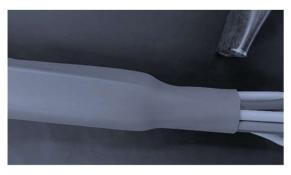
c. Work progressively to the end of the tubing ensuring uniform heat application. This can be achieved by either rotating the assembly or the heat gun. See figure 2. Ensure there is no air entrapment inside.
