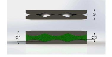
Since the gasket will compress between 10% and 20%, we will require 20% compression at the high points (G2) and 10% at the low points (G1). The greatest gap is therefore 15% of the gasket thickness (G1).
