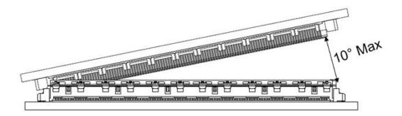
Place one side in and the other side is  $10^{\circ}\,$  Max. upwards and then place the other side in.
