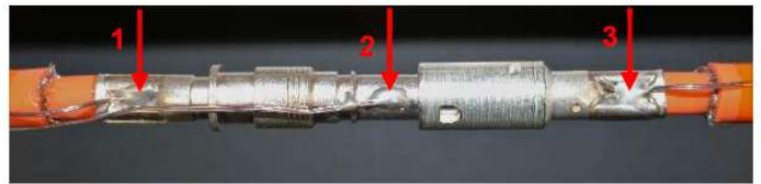
Figure 6 Thermocouple on the crimps and on the pin. Highest temperature value at the pin (2).
