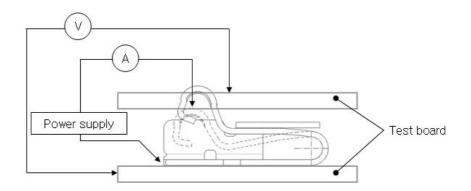
Fig.4 Contact Resistance Measuring Points
