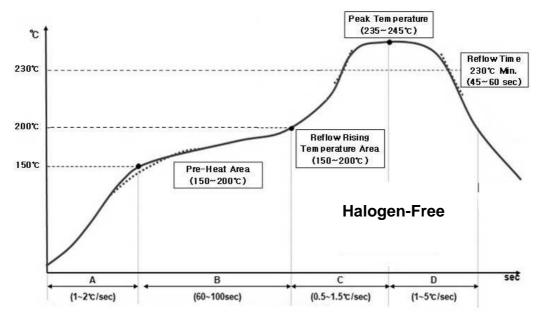
Fig.3 Reflow temperature profile
