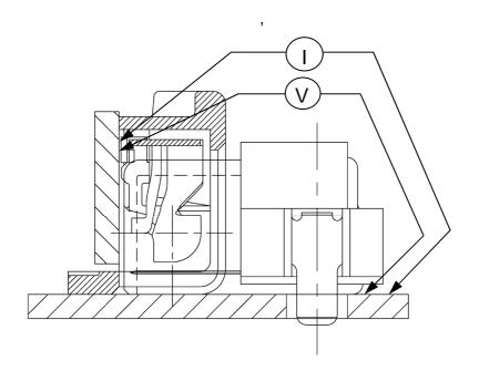
Fig.1 Termination Resistance Measuring Points
