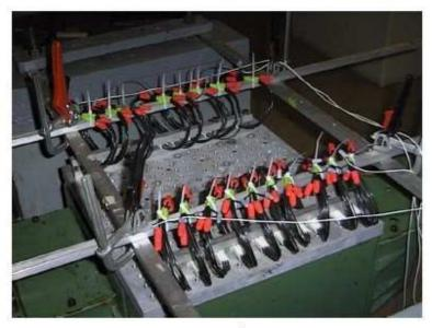
Figure **6**Vibration Mounting Fixture
