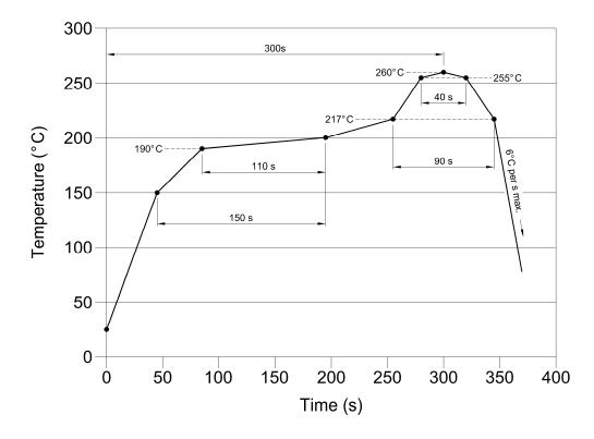
Temperature Profile of Reflow Soldering
