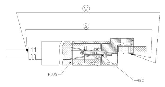
Low Level Contact Resistance Measurement Points Figure 3
