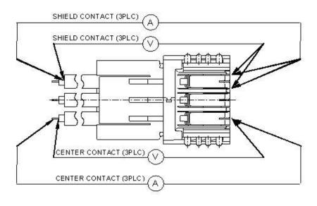
Figure 3 LLCR Measurement Points
