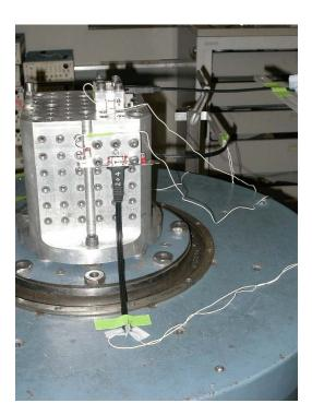
Figure 4 Vibration and Mechanical Shock Mounting Fixture
