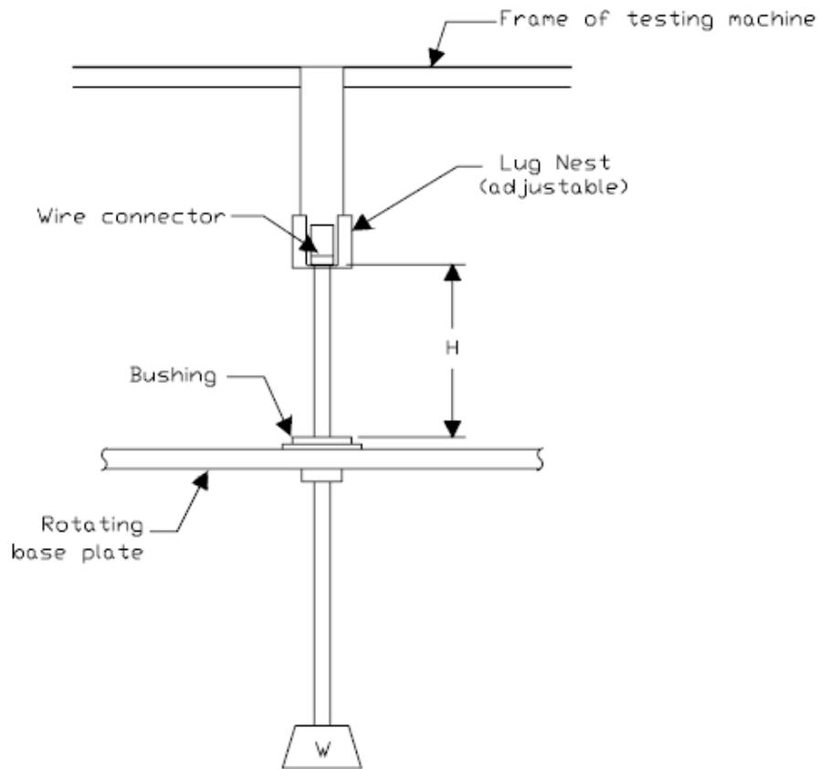
**Figure 6-- Equipment for Secureness test**
