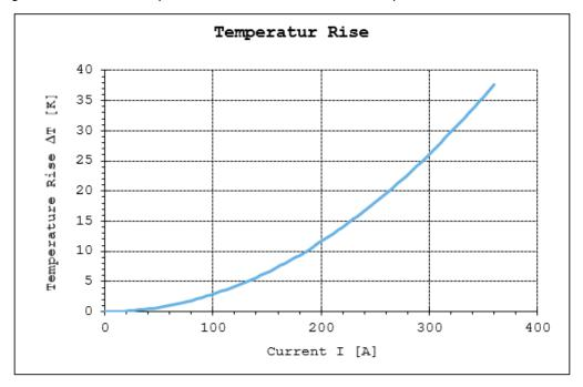
Figure 2. Current & Temperature-rise Curve of TE Crown Clip Junior HC250 Power Connector 2204899
