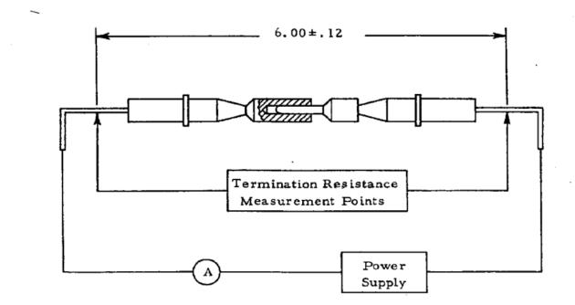
Note: Termination resistance equals millivolts divided by test current less resistance of 6 inches wire.
